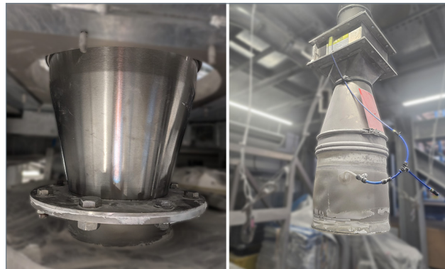
Left: Custom Fabricated Spigot - flange and tapered pipe Right: BFM® Bulk Bag Loader with BFM® Lipped Spigot
