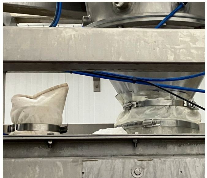
2 different connector types, with jubilee clips, on site
