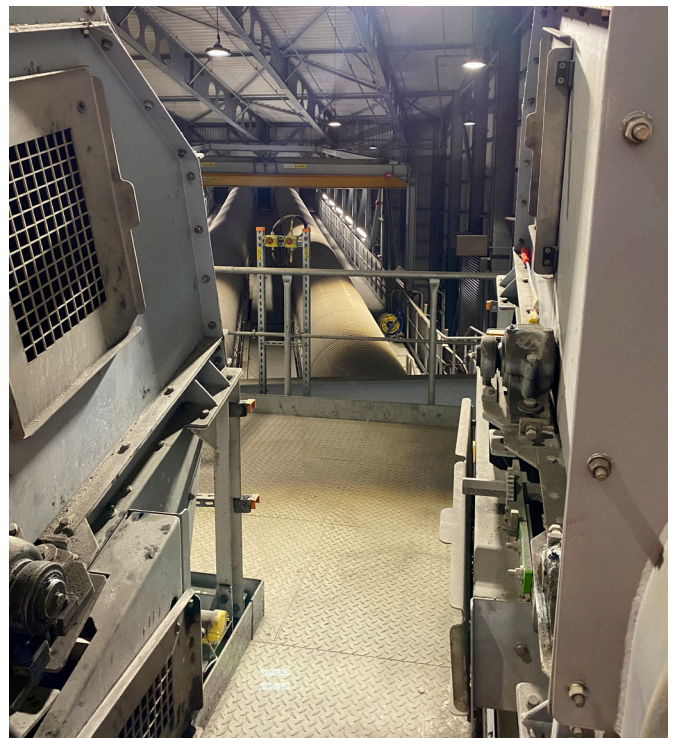
2 belt conveyor streams handling incinerator bottom ash (IBA)
