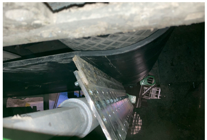
STARCLEAN® secondary cleaner under the main feed belt conveyor
