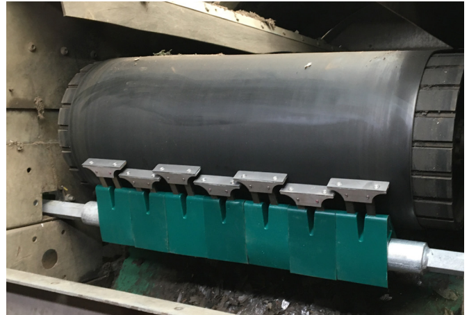
Example of a Starclean Primary Cleaner with 85n Blades
