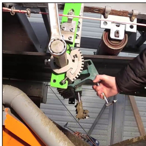
Toolless blade replacement
