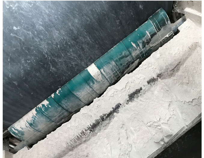
Starclean primary cleaner in operation
