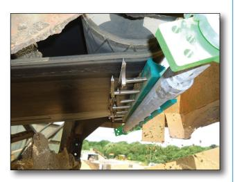
**Our Solution:** Starclean 53sn secondary cleaner with integrated PU primary lip in underbelt location with 800 series quick release tensioner
